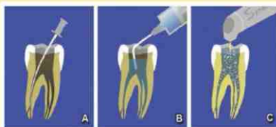
Fig. 1 After root canal enlargement, a sufficient volume and constant flow of irrigant (such as 17% of EDTA) is required to allow a "sonic boom" effect to ripple throughout the root canal system
