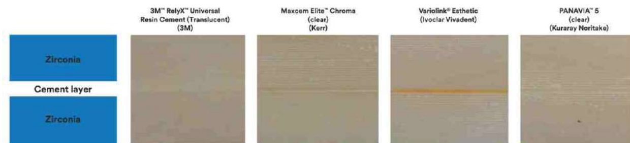
Fig. 14: Discoloration of cement layers after 24 hours of storage in coffee solution. Source: 3M internal data
